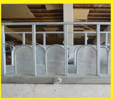
Internal Circular-shaped frames with mass head locking mechanism
