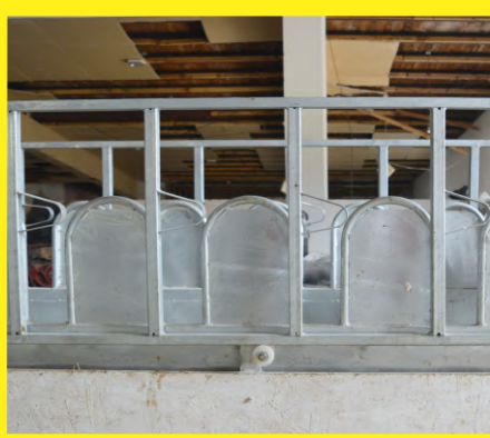
Internal Circular-shaped frames with mass head locking mechanism
