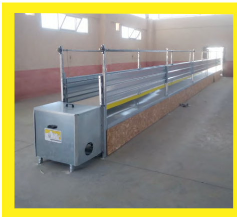
Movable Barriers driven by stainless steel wire rope
