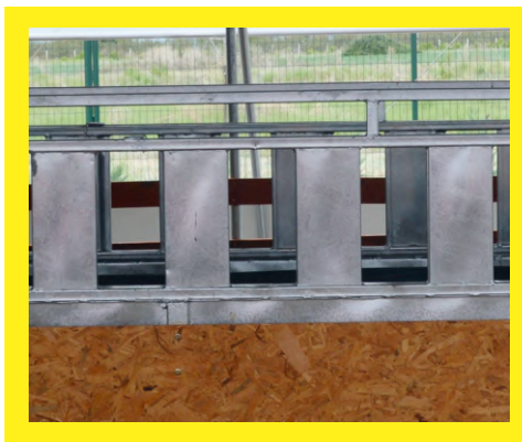
Rectangular-shaped frames with mass head locking mechanism
